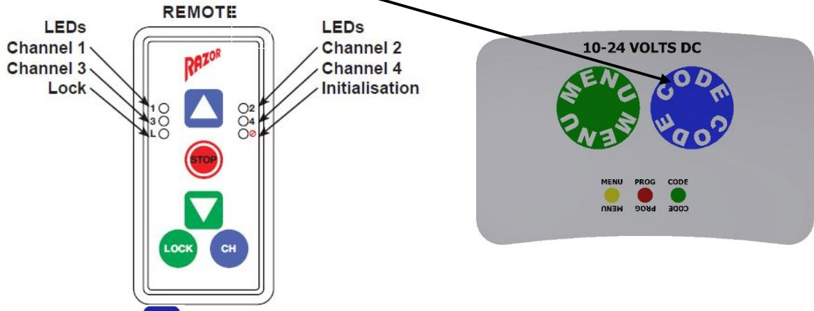
2. Press blue "▲" button on the remote once initially, and then twice. The blue led on receiver keypad will illuminate for 3 seconds (Blue)
